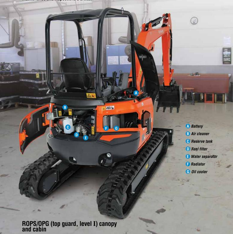
The ROPS/OPG (Top Guard, Level I) canopy and cabin provide protection in the event of accidental rollovers and
