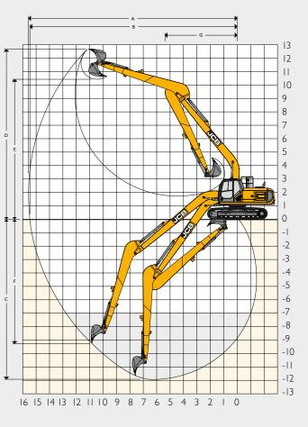
Working dimensions calculated using 980/B0092 GP bucket on Monoboom and T.A.B. and 980/A0391 GP bucket on LR.
